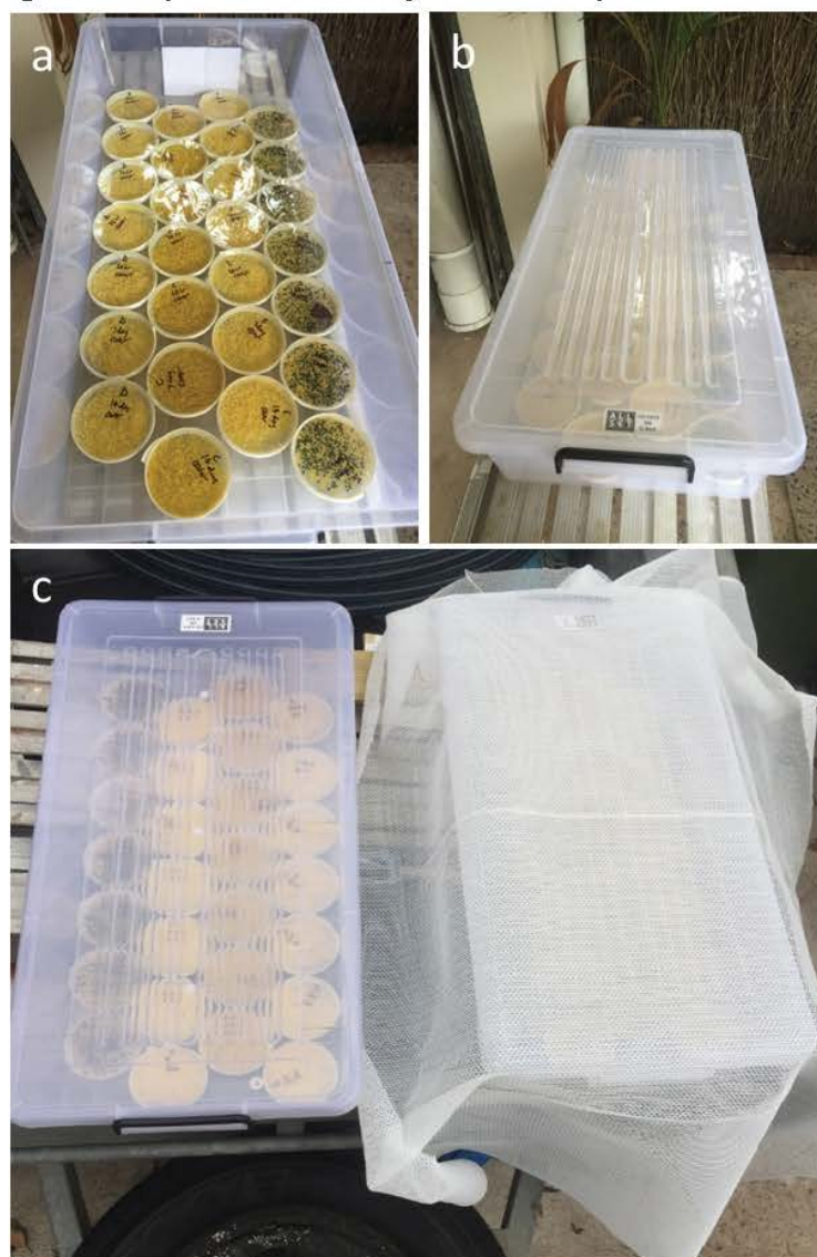
Figure 1: Exposure scenario for ant bait a. Sheltered tub shown without lid b. Sheltered tub with lid in place c. Full sun and shaded tubs with lids and shade cloth in place. NB petri dishes are labelled out to 14 days of exposure but these were adjusted during to the study for a maximum exposure of 8.5 days.
